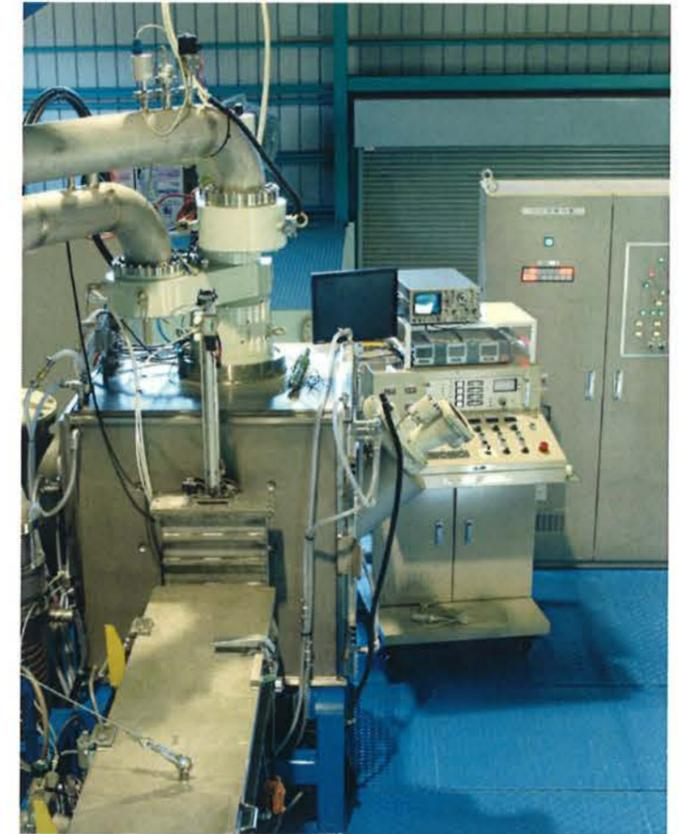
300KW EB 溶解炉
